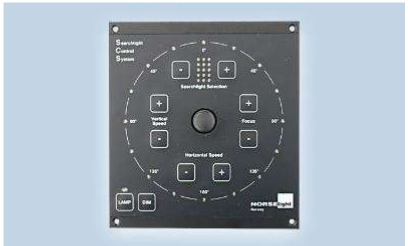
Lamp ON/OFF, positioning, speed control and Searchlight number in use
